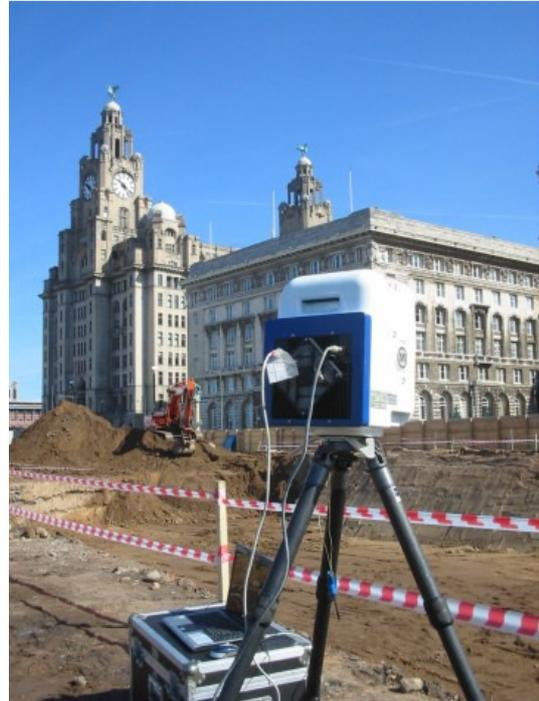
Finally, having excavated a massive proportion of the Liverpool Waterfront, the 3D laser scan images allow the use of GIS and other mapping technology to create a three dimensional model of the waterfront through the ages. This is advantageous as it represents a renewable resource with applications in interpreting the data as well as archiving, publication and potentially also in the “e-learning” forum.
