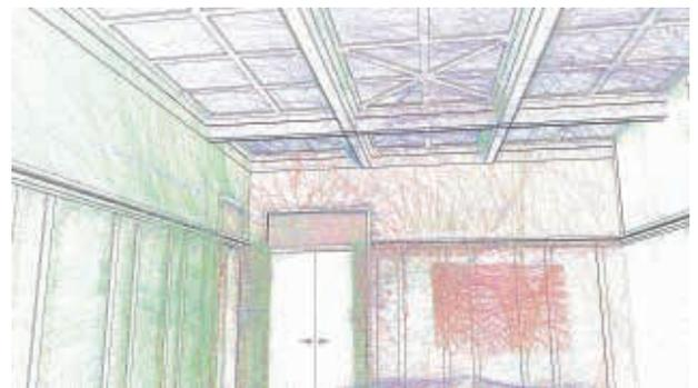
Revit BIM model constructed from GeoSLAM ZEB1 point cloud survey data.
